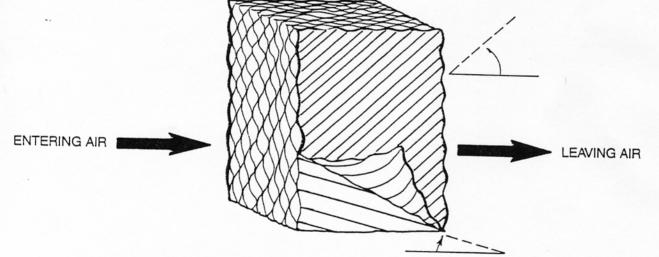
Pads must always be installed with the steeper flute angle sloping down toward the air entering side. The reasoning is simple. The steeper angle puts more water on the hot, dry, dirty side of the pad where it is needed most. It also counteracts the tendency of the air to push the water toward the back of the pad.
